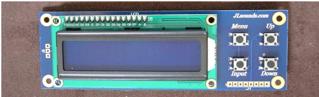
With LCD control board one can select internal settings of the AK4490 DAC IC.
