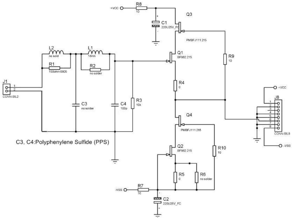
On the PCB board one can design filters from 1<sup>st</sup> to 4<sup>th</sup> order, or the board could be configured as a buffer. The default order is 2<sup>nd</sup>
