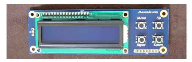
With LCD control board one can select internal settings of the AK4490 DAC IC.
