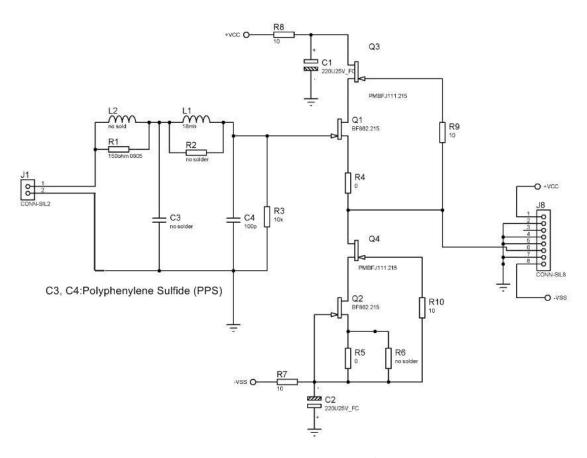
On the PCB board one can design filters from  $1^{st}$  to  $4^{th}$  order, or the board could be configured as a buffer. The default order is  $2^{nd}$
