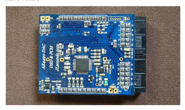
J6, I/O interface – external power supply input for the AK4490 DAC, oscillators and reclock on the I2SoverUSB board 5.2V 0.2A.
